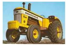
The G1000 wheatland tractor was produced from April 1966 through 1969. During this time frame 821 LP and 2050 diesel wheatland models were produced. Wheatland models differed from row crop models in their fixed tread I-beam front axle, large wrap over rear fenders with operator station front close out panels and lack of available 3pt hitch. The operator boarded the wheatland from the back of the tractor whereas the row
